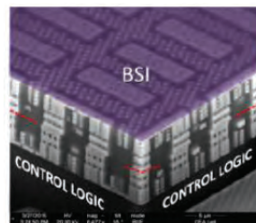
Figure 3: SEM images (TOP view, 3D view) of the 3D assembly including all metal levels of the BSI imager structure. (Dashed lines highlight bonding interface).
