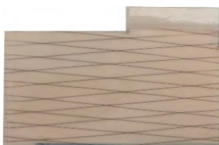
Figure 1: Thermal flexible composite harvester using commercial-grade PVDF and Nitinol wires on both sides used for demonstration (3 x 4.8 cm 2 ).
