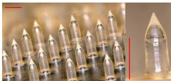
Digital microscopy images of MN-patch fabricated by solvent casting molding method
