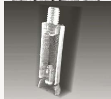
▲ THz tomography of a screw inside a piece of teflon
