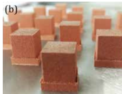
Fig. 7: a) Density map of CuCrZr L-PBF cubes constructed with a 100 µm hatch parameter ; b) Resulting cubes; c) Microstructure of as-built L-PBF CuCrZr sample after a chemical attack in the z direction. After [12].
