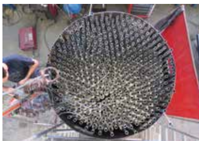
Fig. 4: View of the PCM HS demonstrator [P3] before PCM filling.
