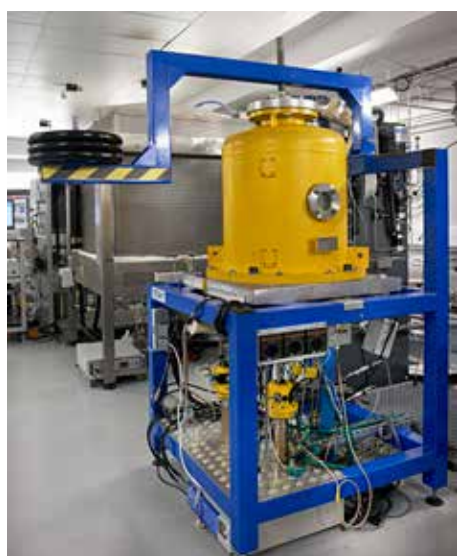
Fig. 1: (a) Photograph of the test rig and (b) scheme of the cell housing for pressurized tests.
