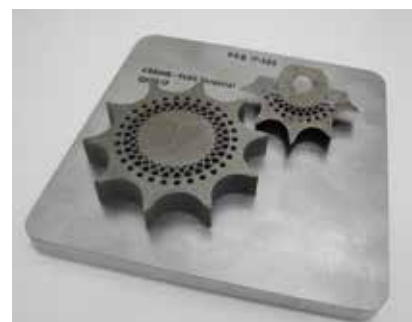
Fig. 9: (a) Electrical and magnetic properties of Fe-Si alloys processed by L-PBF, after A. Krings, IEEE Trans. on Industrial Electronics, Vol 64, Issue 3 (2017) 2405-2414; (b) L-PBF as printed Fe-Si rotor parts, after [15]
