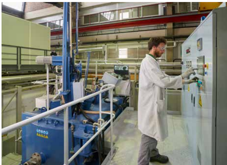
Figure 2: Strip casting equipment for synthesising ferromagnetic alloys at CEA-LITEN.
